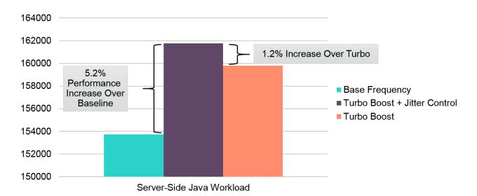
Jitter smoothing is designed to reduce latency by limiting the causes for frequency changes. While throughput performance metrics are impacted by enabling Jitter Control, the removal of latency spikes is critical for workloads that either cannot tolerate latency or have costs associated with computational latencies. When using auto-tuned mode, jitter within the 10-15 usec range caused by frequency changes can be completely eliminated.
